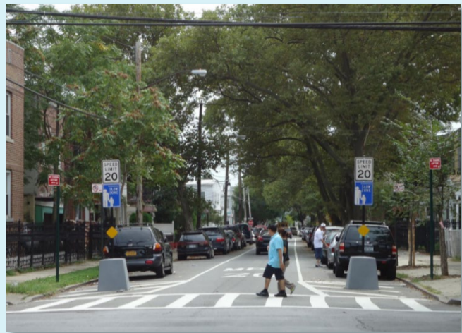
Note: Neighborhood slow zone in New York City. Source: NACTO Urban Street Design Guide .
