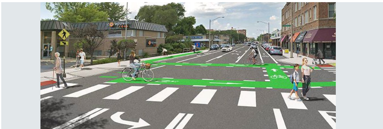
Figure 22. Oak Park, Illinois reduced the number and width of travel lanes to effectively reduce speeding
