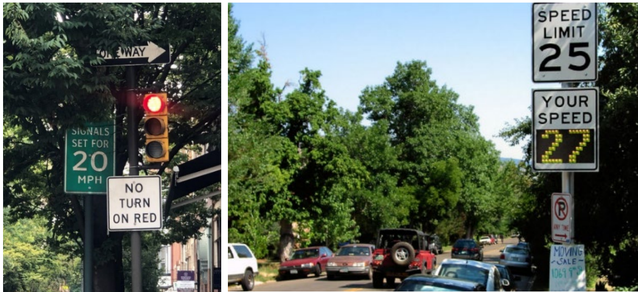
Figure 28. Approaches like signal synchronization (left) and speed feedback sign (right) can raise awareness and help manage speeds
